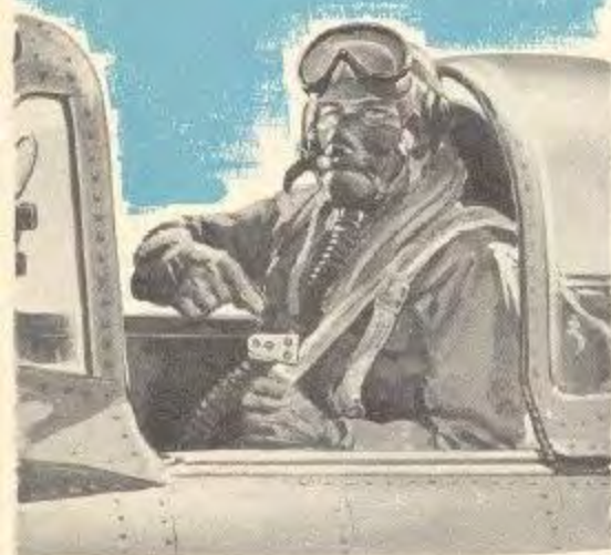
Clip oxygen hose to shoulder harness, not parachute harness, to afford a quick getaway.
