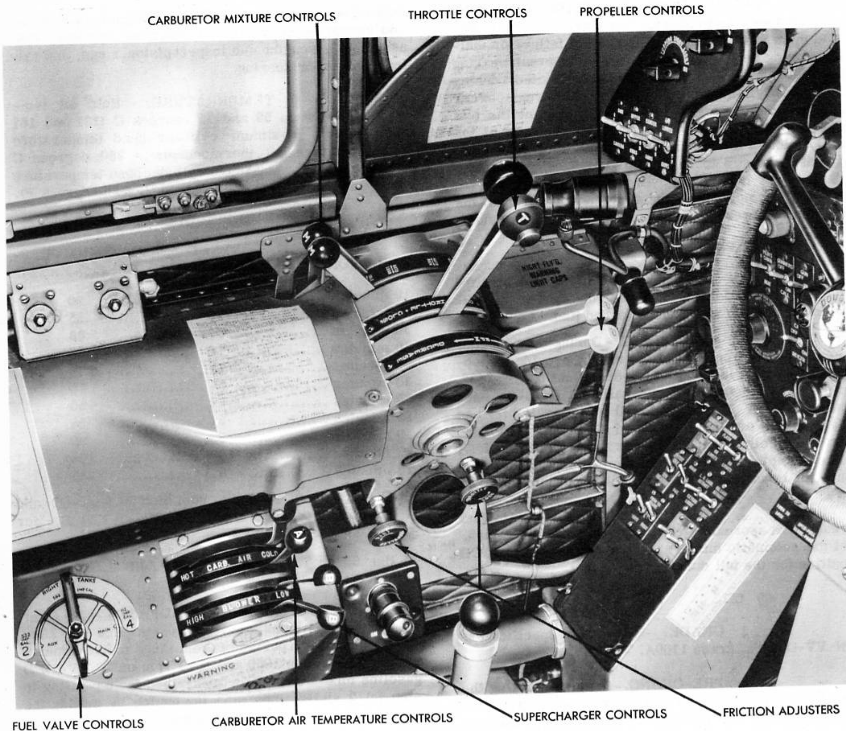
Figure 108 - INSTALLED ENGINE CONTROLS
