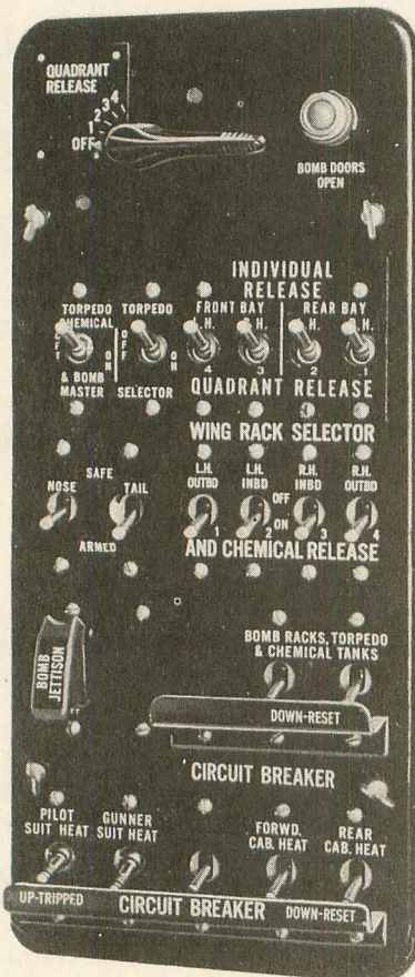
Fig. 42 — Bomb Control Panel
